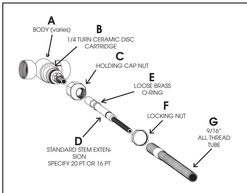
Heavy lever handles require special torque tightening instructions for the spline adapter **Part D**.
